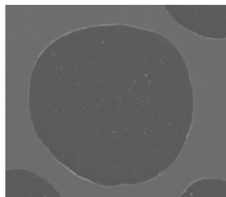
Figure 1. KRYPTOSPHERE LD technology has a very low internal porosity which creates a proppant with high compressive strength and durability.
