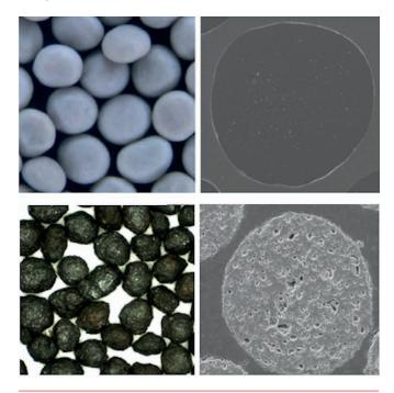
**Figure 4.** KRYTPOSPHERE ceramic proppant technology exhibits exceptionally low internal porosity levels. This results in a proppant with increased compressive strength, high durability and improved crush-resistance.
