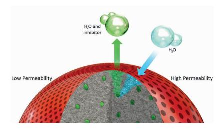
**Figure 2.** GUARD technology features a controlled release technology that ensures a predictable release of the infused chemical in the well only on contact with water. The controlled release technology significantly lengthens treatment life and reduces initial inhibitor washout.
