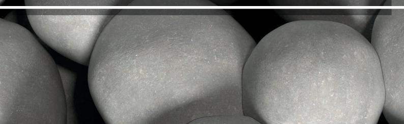
conductivity, contact and durability to enhance production across the full range of low to ultra-high closure stress conditions. Engineered as either a high or low-density ceramic proppant, the proppant portfolio provides high crush-resistance and withstands stress-cycling to ensure fracture conductivity, integrity and connectivity to optimise production.
