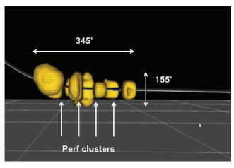
The image on the left from a well in the Bone Springs formation in west Texas was the first one created using electromagnetic imaging, and the image on the right shows reprocessed data from that 8,000-ft deep lateral revealing far more detail. *Source: Paper SPE 184880.*
