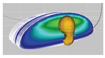
An electromagnetic image of the proppant largely fits into an area, shown in green and turquoise, where a model predicted the most proppant would reside. It also shows significant areas with lower concentrations. Source: Paper SPE 184880.
