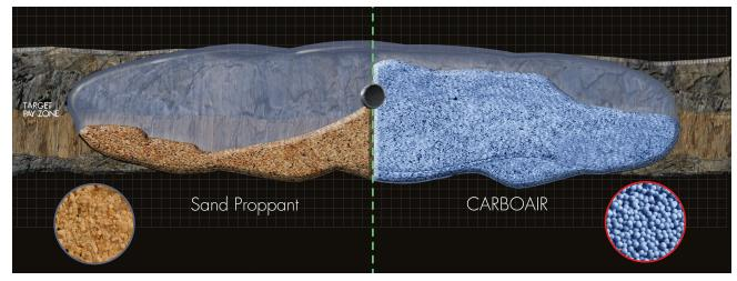
Due to the significantly lower density, 30% less mass of CARBOAIR technology can be used to replace the same volume of sand proppant, thereby reducing the amount of water and chemicals used for the treatment. CARBOAIR technology also provides more coverage across the pay zone, leading to increased production. (Source: Carbo)
