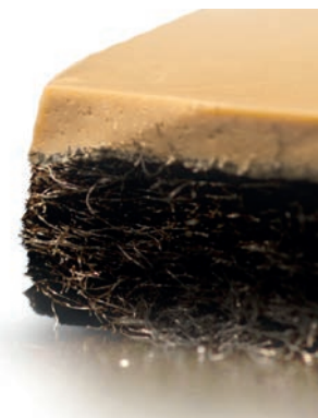
Unlike some providers, our liner thickness specification dictates the actual thickness of the polyurea, never the composite.
