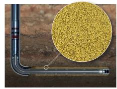
In Alpha/Beta gravel pack completions, CARBOAIR ultra low-density ceramic proppant consistently lowers the height of the Alpha (lower) wave to provide more space and full coverage of the Beta (upper) return wave.
