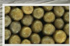
**Control proppant flowback and fines** Reduce effective stress on proppant and prevent proppant flowback with CARBOBOND resin-coating technology. Formulated to be compatible with today's complicated fracturing fluids, the technology is usable in a range of applications.
