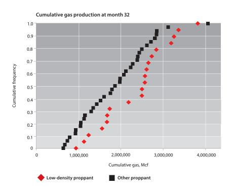
After 32 months of production, low-density ceramic wells produced on average 0.5 Bcf/well more than offset wells containing RCS.
