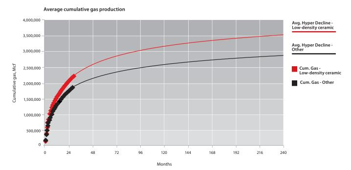
When projecting to 20 years using hyperbolic decline, it is projected that the ceramic proppant wells will produce an incremental 35% more gas than the RCS proppant offset wells. Sources: SPE 134165 "Improving Stimulation Effectiveness – Field Results in the Haynesville Shale" and SPE 160206 "Hydraulic Fracture Design Optimization in Unconventional Reservoirs – A Case History."
