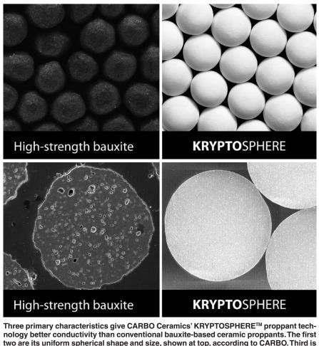
two are its uniform spherical shape and size, shown at top, according to CARBO. Third is improved internal microstructure of the grains (bottom), which don't have the 5 percentplus internal porosity typical of even well-made ceramic proppants, CARBO says.
