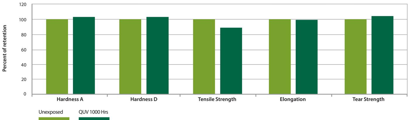
The polyurea spray used in our proprietary liner retains its properties even after years of exposure to UV light and extreme weather conditions. The maximum recommended long-term exposure temperature is 200°F (93°C).
