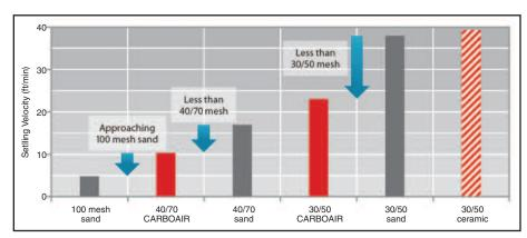
CARBO's CARBOAIR™ ultralow density proppant settles slower than sand or resin-coated sand while offering equal or better conductivity, strength and durability. According to CARBO, these characteristics make the proppant ideal for increasing propped fracture height and length in slickwater or low-gel completions.
