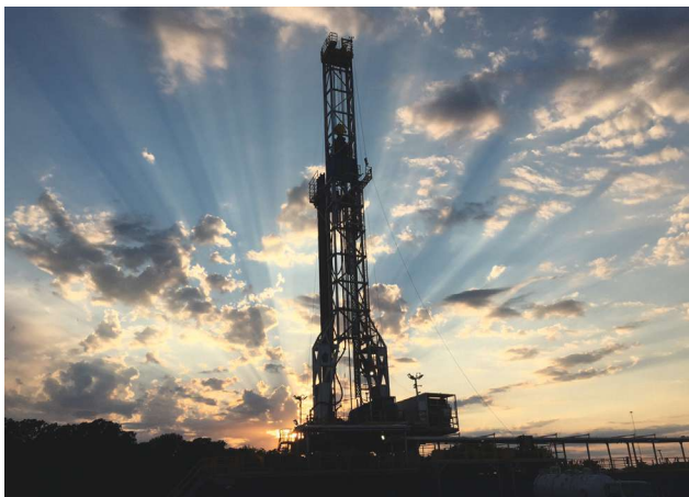
CTF's automated, all-electric triple cyber rig is capable of performing any type of downhole tool and technology drilling test. (Source: Catoosa Test Facility)
