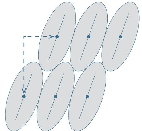
Optimum well placement in low-permeability Wilcox sands of Culebra portion of the field indicates an elliptical drainage pattern characteristic of low-perm hydraulically fractured reservoirs.
