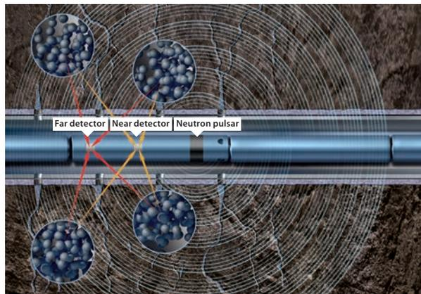
CARBONRT technology enables cost-effective fracture evaluation of ceramic completed wells on a standard neutron logging tools run.
