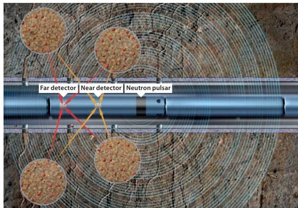
CARBONRT ULTRA technology enables cost-effective fracture evaluation of sand completed wells on a standard neutron logging tools run.
