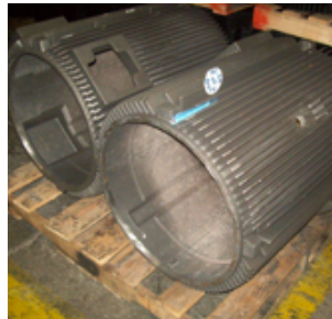
Motor house frames, post-blast
