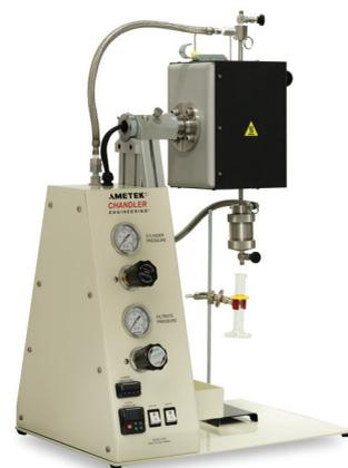
**Chandler Engineering's new Model 4300 Fluid Loss Cell measures the fluid loss properties of muds and cement slurries. (Source: Chandler Engineering)**
