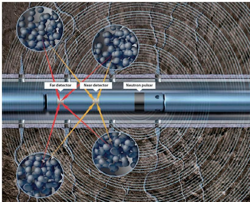
**Figure 1.** The first generation CARBONRT non-radioactive traceable proppant is manufactured with a high thermal neutron capture compound (HTNCC) added uniformly throughout every grain of the host proppant. A standard neutron log run before and after the fracture treatment can then detect the presence of the proppant to accurately measure proppant coverage and fracture height near the wellbore.
