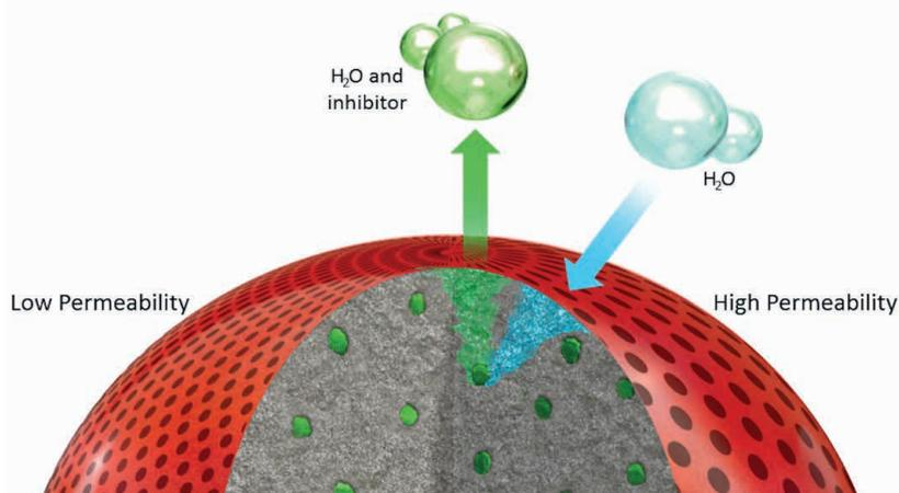
**Figure 2.** GUARD technology features a controlled release technology that ensures a predictable release of the infused chemical in the well only on contact with water. The controlled release technology significantly lengthens treatment life and reduces initial inhibitor washout.
