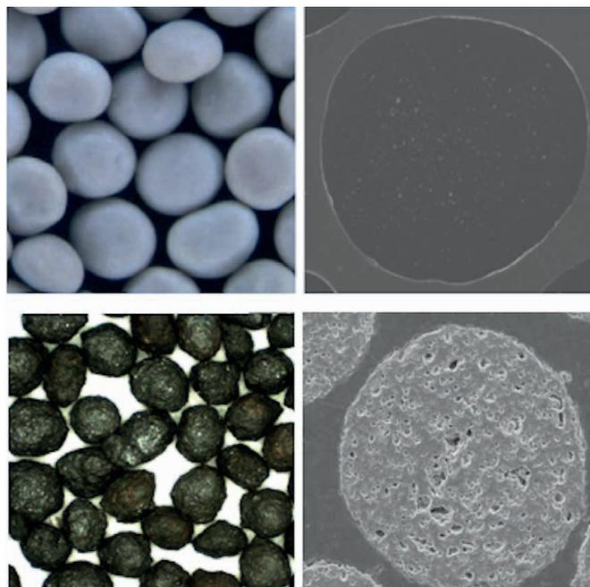
*Figure 4. KRYPTOSPHERE ceramic proppant technology exhibits exceptionally low internal porosity levels. This results in a proppant with increased compressive strength, high durability and improved crush-resistance.*
