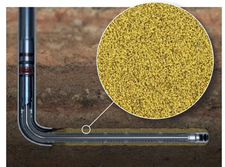
In Alpha/Beta gravel pack completions, CARBOAIR ultra low-density ceramic proppant consistently lowers the height of the Alpha (lower) wave to provide more space and full coverage of the Beta (upper) return wave.
