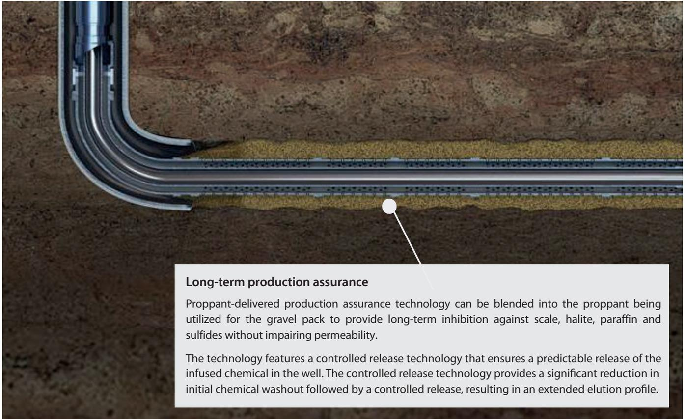
**SCALEGUARD®:** Carbonate and Sulfate scale prevention
