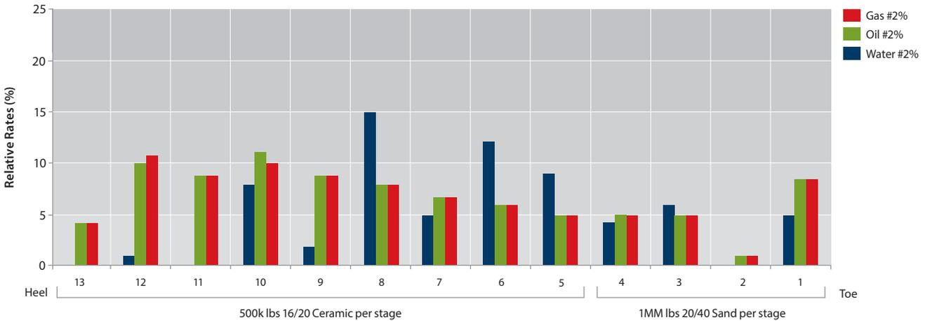
Figure 2: VBA-6E: SPF Performance Evaluation, Normalized Plot
